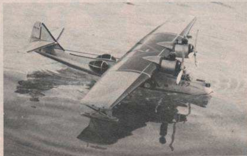
Henry's Consolidated PBV-5A "Catalina" spans only 24" and is powered by a pair of Cox .020 engines. Built in 1958, it is probably the smallest flying twin-engined airplane that we have seen around.
