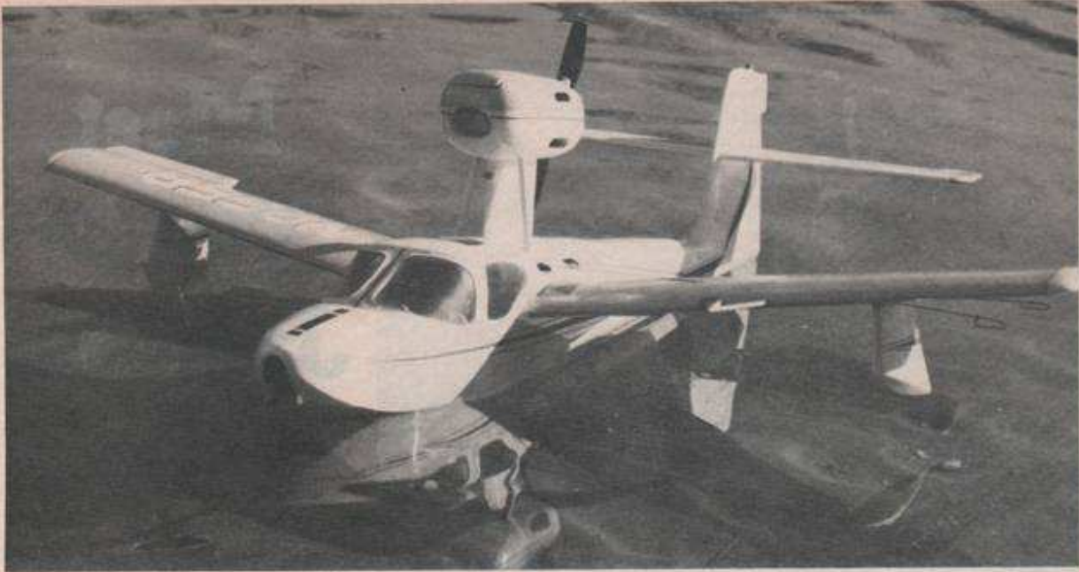
The Piper "Super Cruiser" (opposite top) was built in 1957 from a modified Berkley kit and rides on Edo floats. The span is 36" and it is powered by an Arden .09. The "Colonial Skimmer" (opposite bottom and above) was built a year later also from a modified Berkley kit. It was completely balsa
